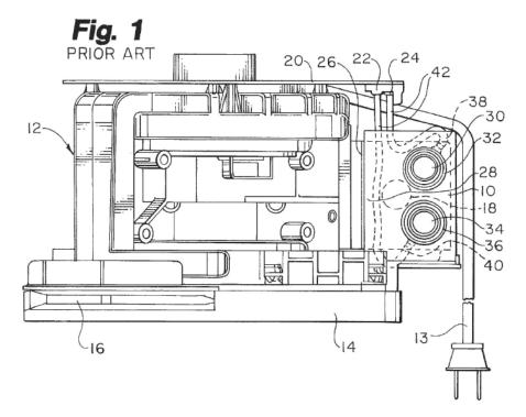
Figure 1 is a front elevational view of prior art valve enclosure assembly 10 coupled to pump 12. *Id.* at 1:13–14, 3:27–28. Air inlet 16 provides inlet air to pump 12, and pressurized air is discharged from pump 12 into prior art valve enclosure assembly 10 through air outlet 18 in the rear face of the valve enclosure assembly. *Id.* at 1:16–20. Front face 28 of prior art valve
