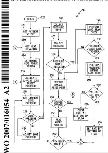
(57) Abstract: A patient support (10, 14) includes a source of pressurized air (64), a bladder (30), a valve (66) in fluid communication with the source of pressurized air (64) and to the bladder (30), a pressure sensor (28) in fluid communication with the bladder (30), and a controller (26) responsive to a pressure signal from the pressure sensor (28). The controller (26) may determine a rate of change of pressure within the bladder (30) and may store historical pressure data.
