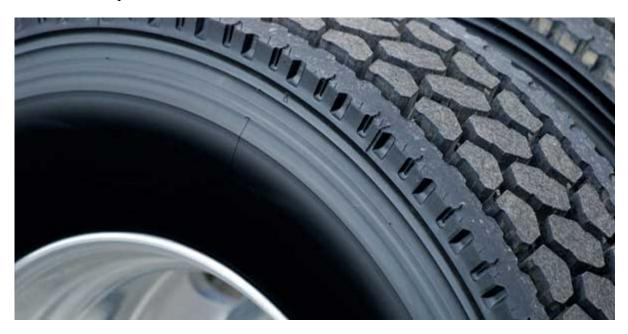
Every fleet determines its recommended tire pressure based on the worst vehicle load. Since loads vary by wheel position, using the load/inflation tables published by any tire manufacturer will determine the proper <u>tire</u> <u>pressure based on the specific load</u>. That is why many fleets have a <u>different air pressure specification</u> for steer versus drive versus trailer tires. Those load/inflation tables are all based on an ambient temperature of 70 degrees F.
