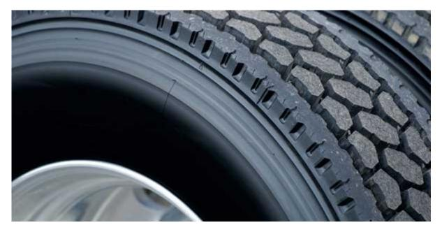
Every fleet determines its recommended tire pressure based on the worst vehicle load. Since loads vary by wheel position, using the load/inflation tables published by any tire manufacturer will determine the proper <u>tire</u> pressure based on the specific load. That is why many fleets have a <u>different air pressure specification</u> for steer versus drive versus trailer tires. Those load/inflation tables are all based on an ambient temperature of 70 degrees F.
