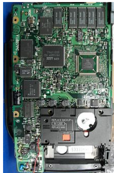
Inside the Apple Newton Messagepad H1000, with back cover removed
