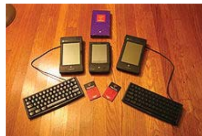
Three Newton MessagePad devices with keyboard and LinearFlash PCMCIA memory card accessories
