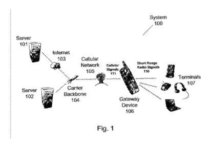
First wireless devices (terminals 107) are provided means for accessing a data network such as Internet 103 over a cellular network 105 using gateway device 106.
