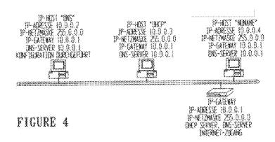
The gateway device operates as a DHCP server if it determines such is necessary in order to allocate IP addresses in the local network. *Id.* at col. 4 II. 34-56.
