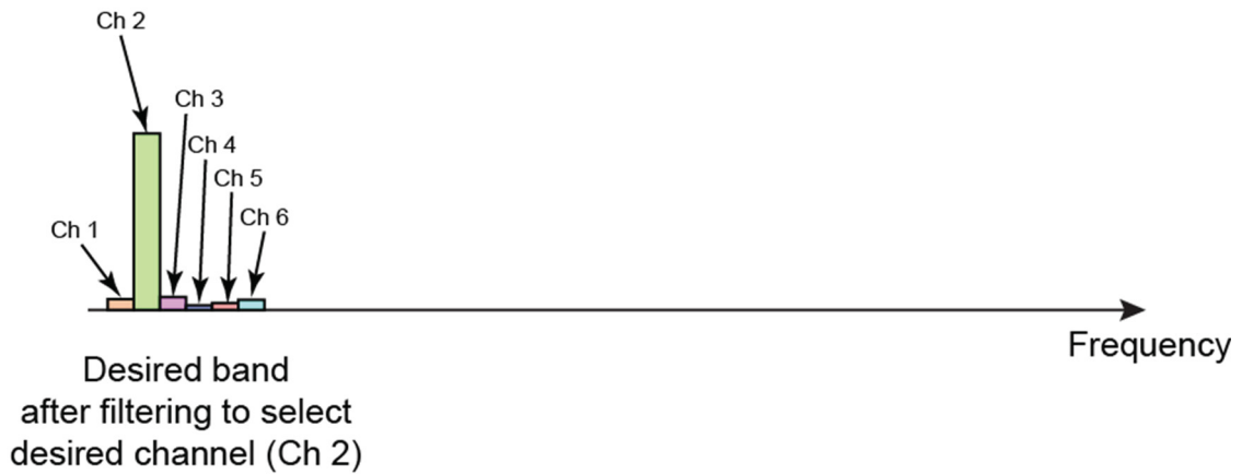
Figure 5. Additional filters, such as a low-pass filter, further refine the signal to select the specific carrier of interest (Ch 2 in this illustration).
