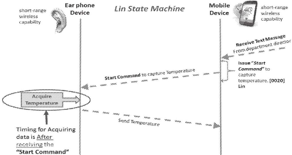
Lin : Timing for Acquiring data is After receiving the "Start Command" from the Mobile device
