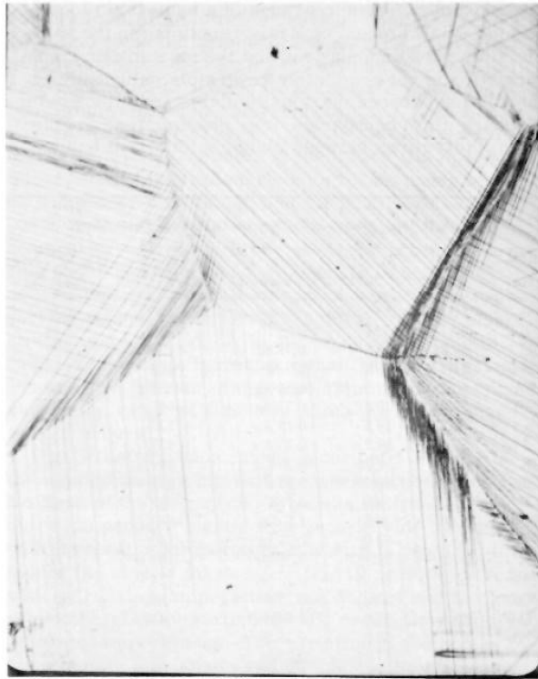
Fig. 10—Martensite plates formed by elastic deformation in alloy A. Magnification 80 times.
