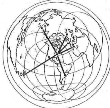
azimuthal equidistant projection, centered on Washington, D.C.: 1 London, 2 Algiers, 3 Moscow, 4 Rio de Janeiro, 5 Tokyo, 6 Auckland
