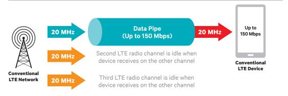
LTE device receives only on one radio channel with maximum data speed limited by radio channel bandwidth
