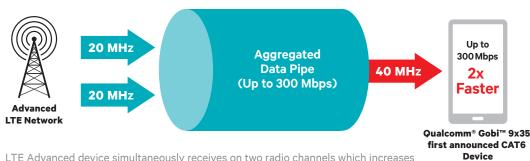
LTE Advanced device simultaneously receives on two radio channels which increases user data rates and reduces latency (faster network response time) as compared to conventional LTE devices
