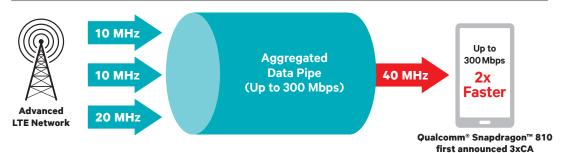
LTE Advanced device simultaneously receives on three radio channels which increases user data rates and reduces latency (faster network response time) as compared to
