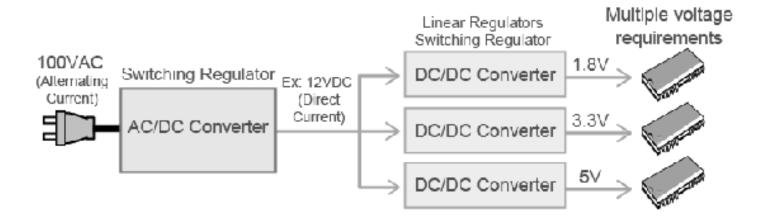
A device that stabilizes the voltage using a DC-DC converter is referred to as a voltage regulator.
