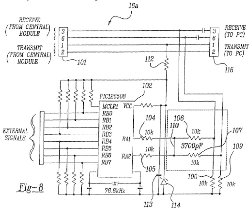
Figure 8 shows resistor 112 connected on a bus between the central module (not depicted) at connector 101 and a PC (not depicted) connected at connector 116. *See* Ex. 1001, 8:22–31, Fig. 4 (showing remote module 16a connected to PC 3a on one side and connected to central module 15a on another side via connectors and a bus). Although the Specification describes resistor circuitry 112 as part of a central module (Ex. 1001, 3:65–67), clearly
