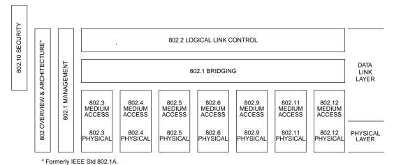
This family of standards deals with the Physical and Data Link layers as defined by the International Organization for Standardization (ISO) Open Systems Interconnection Basic Reference Model (ISO 7498: 1984). The access standards define several types of medium access technologies and associated physical media, each appropriate for particular applications or system objectives. Other types are under investigation.
