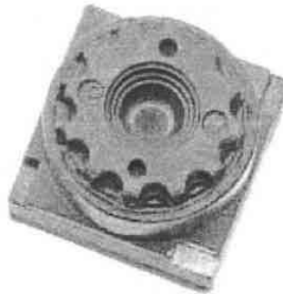
Fig.1: This 3.6 \mu m pixel VGA camera module is 6.05 x 6.05 x 4.5 mm. The most critical dimension is the 4.5 mm axial length.
