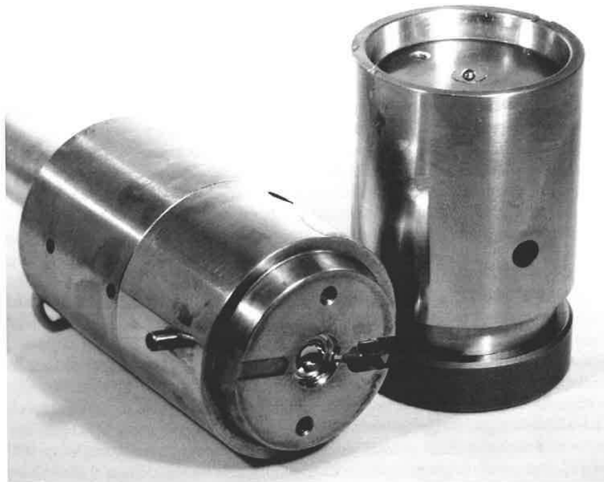
Figure 3.8 Inserted cavity set for injection mold. Note the tapers on the two halves, which interlock the cavity set. (Photograph courtesy of Alan Symmons.)
