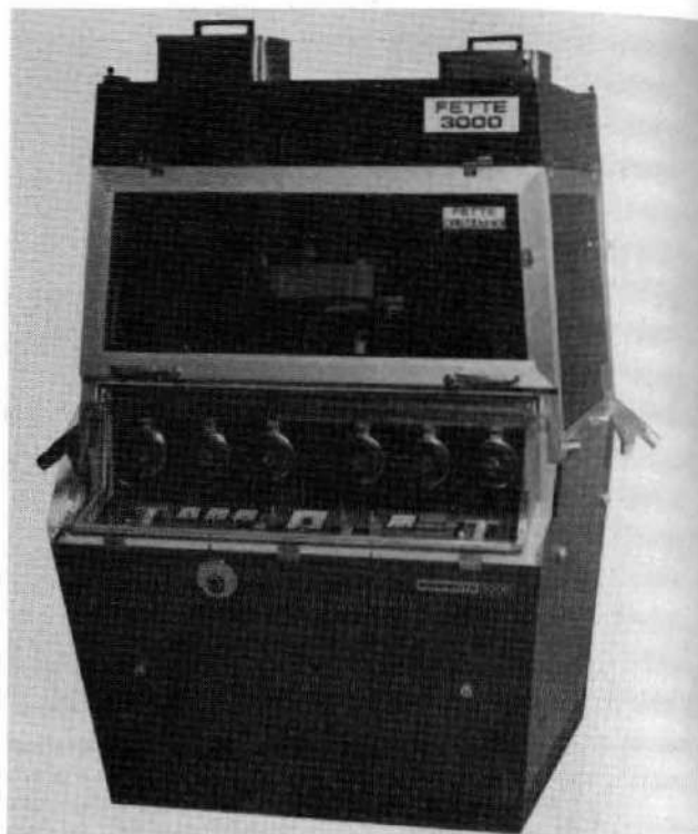
Figure 45-32. Fette Perfecta 3000 high-speed tablet press with pressing compartment completely sealed off from outside environment, making cross-contamination impossible (courtesy, Raymond Auto).
