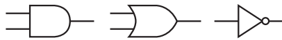
FIGURE B.2.1 Standard drawing for an AND gate, OR gate, and an inverter, shown from left to right. The signals to the left of each symbol are the inputs, while the output appears on the right. The AND and OR gates both have two inputs. Inverters have a single input.
