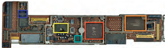
FIGURE 1.8 The logic board of Apple iPad 2 in Figure 1.7 . The photo highlights five integrated circuits. The large integrated circuit in the middle is the Apple A5 chip, which contains a dual ARM processor cores that run at 1 GHz as well as 512 MB of main memory inside the package. Figure 1.9 shows a photograph of the processor chip inside the A5 package. The similar sized chip to the left is the 32 GB flash memory chip for non-volatile storage. There is an empty space between the two chips where a second flash chip can be installed to double storage capacity of the iPad. The chips to the right of the A5 include power controller and I/O controller chips. (Courtesy iFixit, www.ifixit.com )
