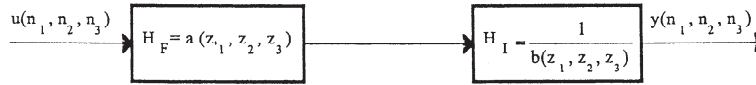
Figure 1. Block diagram of the direct form I realization of a 3-D IIR digital filter.
