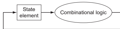
FIGURE 4.4 An edge-triggered methodology allows a state element to be read and written in the same clock cycle without creating a race that could lead to indeterminate data values. Of course, the clock cycle still must be long enough so that the input values are stable when the active clock edge occurs. Feedback cannot occur within one clock cycle because of the edge-triggered update of the state element. If feedback were possible, this design could not work properly. Our designs in this chapter and the next rely on the edge-triggered timing methodology and on structures like the one shown in this figure.
