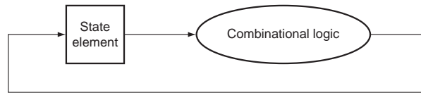
FIGURE B.7.3 An edge-triggered methodology allows a state element to be read and written in the same clock cycle without creating a race that could lead to undetermined data values. Of course, the clock cycle must still be long enough so that the input values are stable when the active clock edge occurs.
