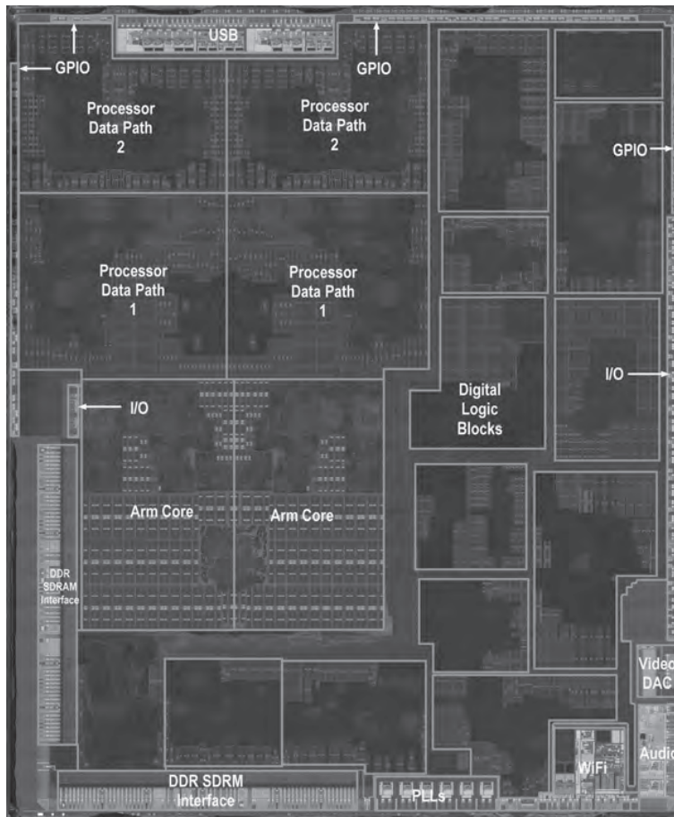
FIGURE 1.9 The processor integrated circuit inside the A5 package. The size of chip is 12.1 by 10.1 mm, and it was manufactured originally in a 45-nm process (see Section 1.5). It has two identical ARM processors or cores in the middle left of the chip and a PowerVR graphical processor unit (GPU) with four datapaths in the upper left quadrant. To the left and bottom side of the ARM cores are interfaces to main memory (DRAM). (Courtesy Chipworks, www.chipworks.com )
