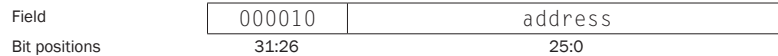
FIGURE 4.23 Instruction format for the jump instruction (opcode = 2). The destination address for a jump instruction is formed by concatenating the upper 4 bits of the current PC + 4 to the 26-bit address field in the jump instruction and adding 00 as the 2 low-order bits.
