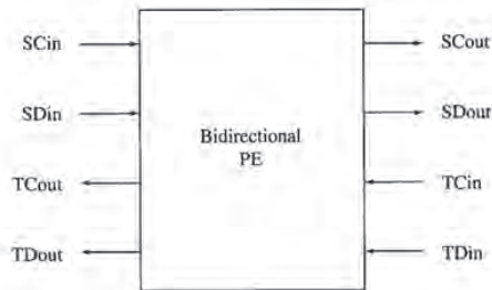
FIGURE 8.6 Processing Element for Bidirectional Array
