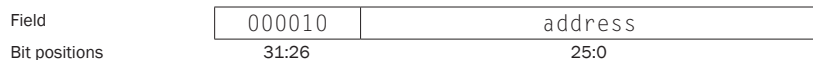
FIGURE 4.23 Instruction format for the jump instruction (opcode = 2). The destination address for a jump instruction is formed by concatenating the upper 4 bits of the current PC + 4 to the 26-bit address field in the jump instruction and adding 00 as the 2 low-order bits.
