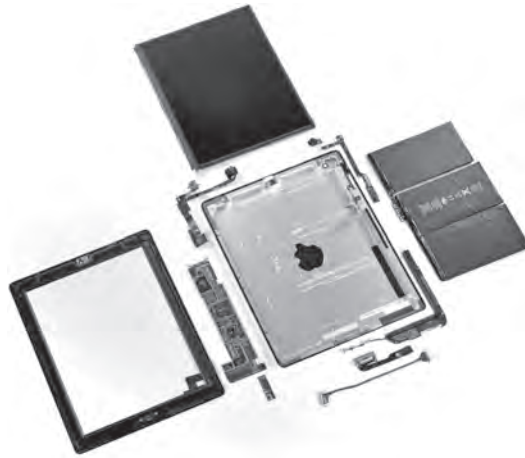
FIGURE 1.7 Components of the Apple iPad 2 A1395. The metal back of the iPad (with the reversed Apple logo in the middle) is in the center. At the top is the capacitive multitouch screen and LCD display. To the far right is the 3.8 V, 25 watt-hour, polymer battery, which consists of three Li-ion cell cases and offers 10 hours of battery life. To the far left is the metal frame that attaches the LCD to the back of the iPad. The small components surrounding the metal back in the center are what we think of as the computer; they are often L-shaped to fit compactly inside the case next to the battery. Figure 1.8 shows a close-up of the L-shaped board to the lower left of the metal case, which is the logic printed circuit board that contains the processor and the memory. The tiny rectangle below the logic board contains a chip that provides wireless communication: Wi-Fi, Bluetooth, and FM tuner. It fits into a small slot in the lower left corner of the logic board. Near the upper left corner of the case is another L-shaped component, which is a front-facing camera assembly that includes the camera, headphone jack, and microphone. Near the right upper corner of the case is the board containing the volume control and silent/screen rotation lock button along with a gyroscope and accelerometer. These last two chips combine to allow the iPad to recognize 6-axis motion. The tiny rectangle next to it is the rear-facing camera. Near the bottom right of the case is the L-shaped speaker assembly. The cable at the bottom is the connector between the logic board and the camera/volume control board. The board between the cable and the speaker assembly is the controller for the capacitive touchscreen. (Courtesy iFixit, www.ifixit.com )
