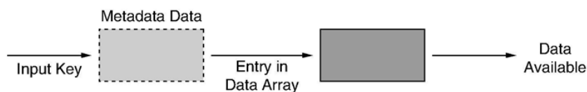
FIGURE Ov.2: An idealized cache lookup. A cache is logically comprised of two elements: the data array and some management information that indicates what is in the data array (labeled “metadata”). Note that the key information may be virtual, i.e., data addresses can be embedded in the software using the cache, in which case there is no explicit key lookup, and only the data array is needed.
