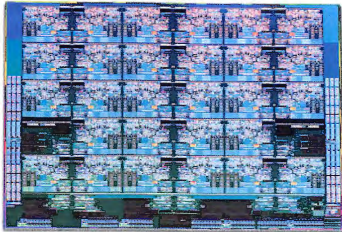
Figure 1.14 Photograph of an Intel Skylake microprocessor die, which is evaluated in Chapter 4.
