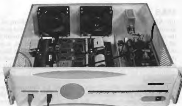
FIGURE 34.12 ■ FPX modules integrated in a rack-mount chassis.
