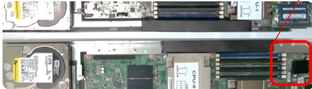
Data Center Server (1U, ½ width)
