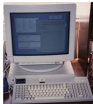
Sun SPARCstation 1+ "pizzabox", 25 MHz SPARC processor, early 1990s
