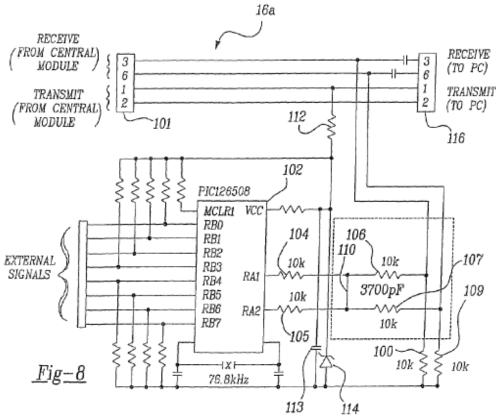
Figure 8 shows resistor 112 connected on a bus between the central module (not depicted) at connector 101 and a PC (not depicted) connected at connector 116. *See* Ex. 1001, 8:22–31, Fig. 4 (showing remote module 16a connected to PC 3a on one side and connected to central module 15a on another side via connectors and a bus). Although the Specification describes resistor circuitry 112 as part of a central module (Ex. 1001, 3:65–67), clearly
