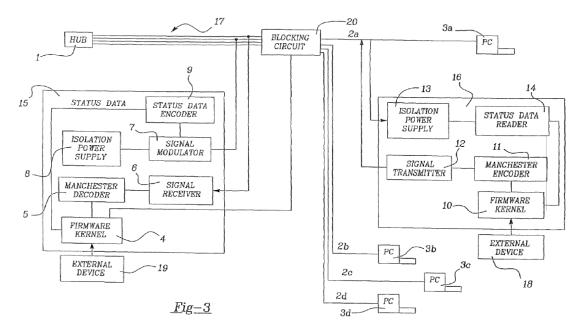
Ex. 1001, Fig. 3. Figure 3 portrays isolation power supply 8 in central module 15, which supplies direct current (DC) to current loops 2a–2d, personal computers (PCs) 3a–3d, and remote module 16a. *See id.* at 5:33–35, Figs. 3, 4.
