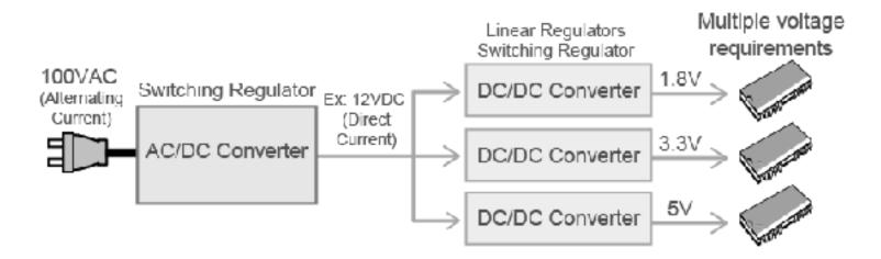
A device that stabilizes the voltage using a DC-DC converter is referred to as a voltage regulator.
