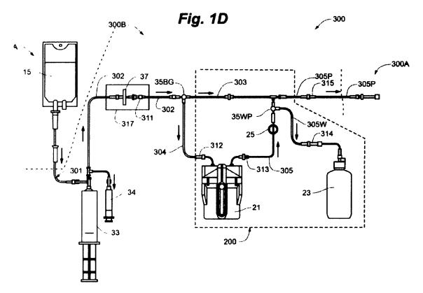
The specification also states that "circuit **300** [can be] expanded to include elements for an automated collection of eluate samples for activity measurements, via the on board dose calibrator." *See id.* at 8:13-16. The specification explains that "a sample collection reservoir
