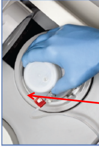
Figure 7, Waste Bottle in Waste Well
