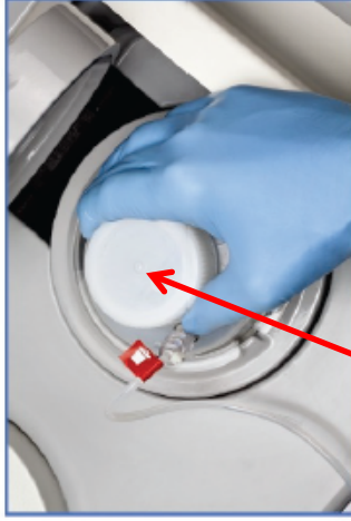
Figure 7, Waste Bottle in Waste Well
