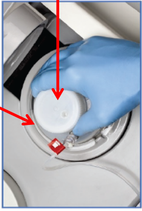
Figure 7, Waste Bottle in Waste Well
