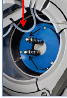
Figure 4, Generator Metal Caps
