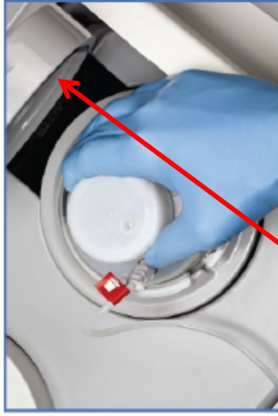
Figure 7, Waste Bottle in Waste Well
