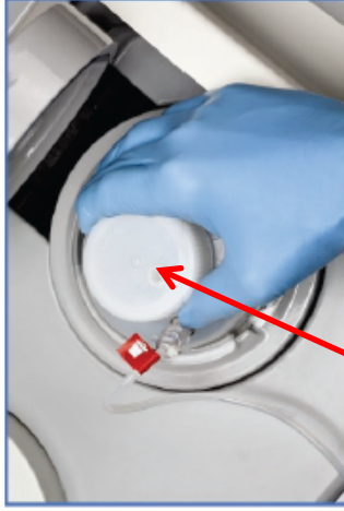
Figure 7, Waste Bottle in Waste Well
