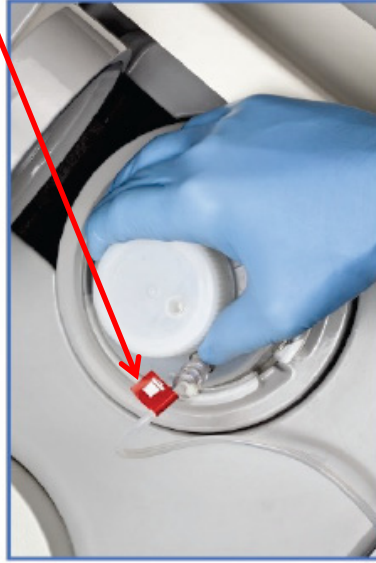
Figure 7, Waste Bottle in Waste Well
