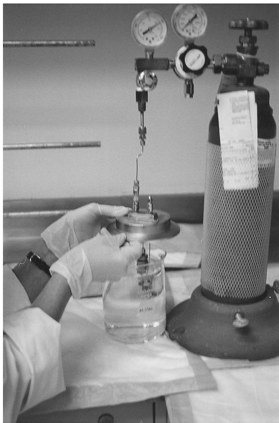
Fig. 3. Leak test of the generator column. The generator column is leak tested by capping the outlet line of the column and passing a static pressure of 50 psi of argon through the column. The generator column is immersed in a beaker containing 1 liter of sterile water. If a leak occurs, argon bubbles will be observed in the water.
