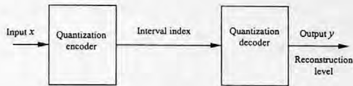
FIGURE 2.14 A two-stage model of quantization.
