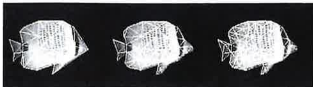
FIGURE 11 Example of a progressive geometry (mesh) construction by successive refinements from left to right.
