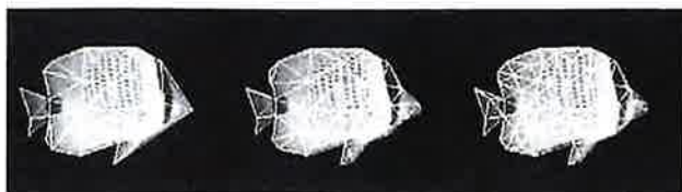
FIGURE 11 Example of a progressive geometry (mesh) construction by successive refinements from left to right.
