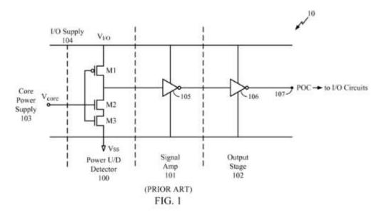
Figure 1 "is a circuit diagram illustrating a conventional POC system for multiple supply voltage devices" which is identified as being prior art. *Id.* at 4:18–19, Fig. 1.
