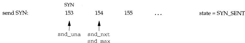
Figure 28.31 Send sequence space when SYN is sent for self-connect.
