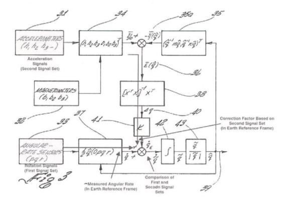
12. <u>1(k)</u> "said resultant angles in the spatial pointer reference frame of the resulting deviation of the six- axis motion sensor module of the 3D pointing device are obtained under said dynamic environments"
