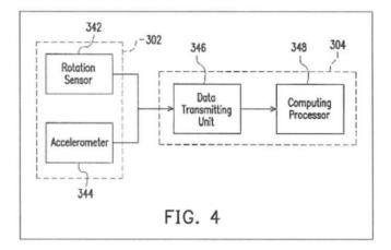
The '438 Patent discloses that in order to calculate deviation angles of the device, the rotation sensor (e.g., gyroscope) generates a set of angular velocity
