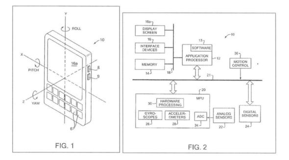
Nasiri discloses that the pointing device, the handheld device, is a 3D device that is capable of facilitate interaction based on "sensing rotational rate around at least three axes and linear acceleration along at least three axes." *Id.*, Abstract, 34:58-60. FIG. 1 shows that the device 10 can rotate in the yaw, pitch and roll angles. *Id.*, FIG. 1.
