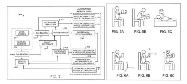
Sachs discloses a system for producing augmented data for recognizing motion gestures using both the first (gyroscopes data) and the second (acceleration data) signal sets, as shown FIG. 7. *Id.*, ¶0062, FIG. 7. Sachs discloses the determination of the resultant angle by showing the rotation matrix and quaternion as representing the orientation of the device.
