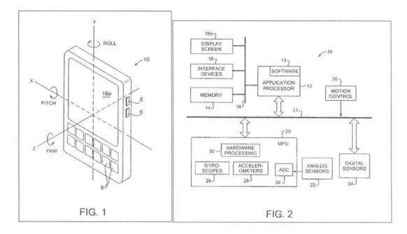
Nasiri discloses that the pointing device, the handheld device, is a 3D device that is capable of facilitate interaction based on "sensing rotational rate around at least three axes and linear acceleration along at least three axes." *Id.*, Abstract,
