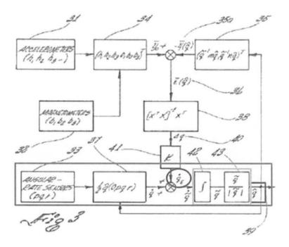
Bachmann describes that when the computations are done in a discrete time system, the predicted value of q is given by equation 16, which clearly shows that the next discrete value of q is determined by the least squares filtered difference " $\Delta q$  (full)" times the time interval between the samples plus the measured angular rate time the time interval. Ex.1007, 11:12-20.
