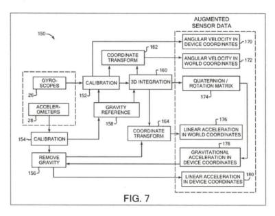
Sachs, incorporated into Nasiri, discloses "the measured state includes a measurement of said second signal set." Sachs discloses accelerometers 28 generates acceleration data as part of the augmented data for device 10. *Id.*, ¶0062. The coordinate transform block 164 receives calibrated linear acceleration data
