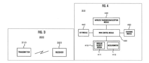
Song also discloses that angular velocity sensor 11 measures the angular velocity data, the first data set, and accelerometer 412 measures the acceleration data, the second data set. *Id.*, ¶¶0042-43.
