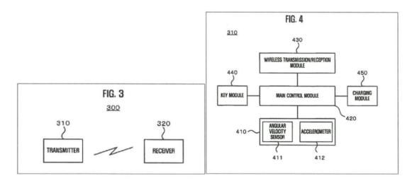
Song discloses that angular velocity sensor 11 measures the angular velocity data, the first data set, and accelerometer 412 measures the acceleration data, the second data set. *Id.*,  $\P$  0042-43.
