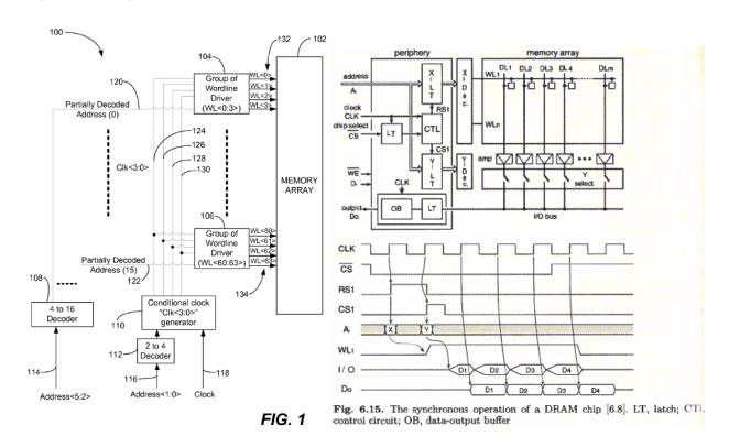
6. In the embodiment in Fig. 1 of the '002 patent, the clock input could be supplied with any type of clock signal—e.g., a periodic clock signal, a non-
