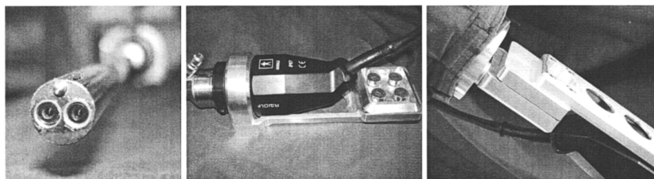
Figure 5. Endoscopic stereo camera with customized magnetic adapter.
