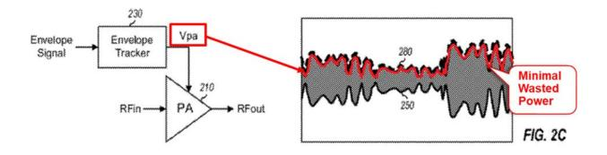
By employing envelope tracking to produce a PA power supply Vpa, represented in plot 280, the "supply voltage closely tracks the envelope [250] of the RFout signal over time." Ex. 1301, 4:21-27. This maximizes PA efficiency by minimizing the difference between Vpa and RFout over time, which results in less wasted power. *Id.* at 4:27-32.
