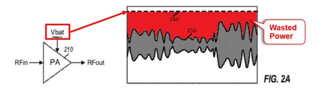
Fig. 2A illustrates using a battery voltage (Vbat) to supply PA 210, which provides an RFout signal as an amplified version of RFin. Ex. 1301, 4:1-3. RFout has a time-varying envelope illustrated by plot 250, which is juxtaposed with voltage Vbat 260. Vbat remains higher than the largest amplitude of RFout's envelop in
