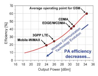
Fig. 1. Efficiencies of PA for various applications
