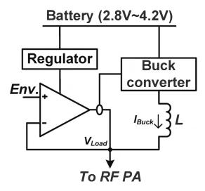
Fig. 5. Battery-to-5V boosting PA supply modulator.
