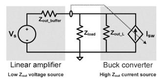
Fig. 4. Simplified block diagram of a hybrid switching amplifier.
