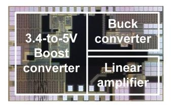
Fig. 8. Microphotograph of the fabricated boosting supply modulator.
