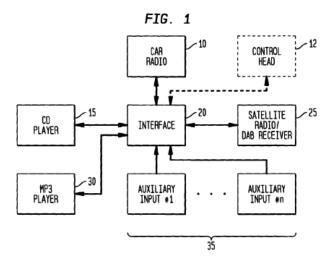
Figure 1 illustrates an embodiment integrating a CD player, a MP3 player, a satellite radio or DAB receiver, and a number of auxiliary input sources with a car stereo. *Id.* at 3:12–13. As shown in the above Figures, central to the '786 patent is an "interface" positioned between the car stereo and the audio device(s) and auxiliary input(s) being integrated.
