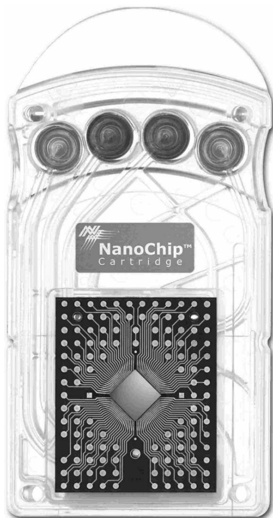
Fig. 5. Nanochip™ Cartridge with microfluidic channels for sample manipulation. Figure courtesy of Nanogen Inc., San Diego, CA.
