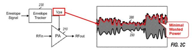
By employing envelope tracking to produce a PA power supply Vpa, represented in plot 280, the "supply voltage closely tracks the envelope [250] of the RFout signal over time." Ex. 1001, 4:21-27. This maximizes PA efficiency by minimizing the difference between Vpa and RFout over time, which results in less wasted power. *Id.* at 4:27-32.
