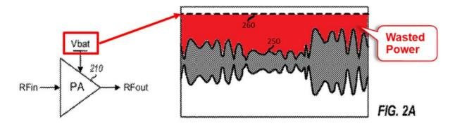
Fig. 2A illustrates using a battery voltage (Vbat) to supply PA 210, which provides an RFout signal as an amplified version of RFin. Ex. 1001, 4:1-3. RFout has a time-varying envelope illustrated by plot 250, which is juxtaposed with voltage Vbat 260. Vbat remains higher than the largest amplitude of RFout's
