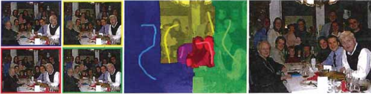
Figure 9.16 Photomontage (Agarwala, Dontcheva, Agrawala et al. 2004) © 2004 ACM. From a set of five source images (of which four are shown on the left), Photomontage quickly creates a composite family portrait in which everyone is smiling and looking at the camera (right). Users simply flip through the stack and coarsely draw strokes using the designated source image objective over the people they wish to add to the composite. The user-applied strokes and computed regions (middle) are color-coded by the borders of the source images on the left.
