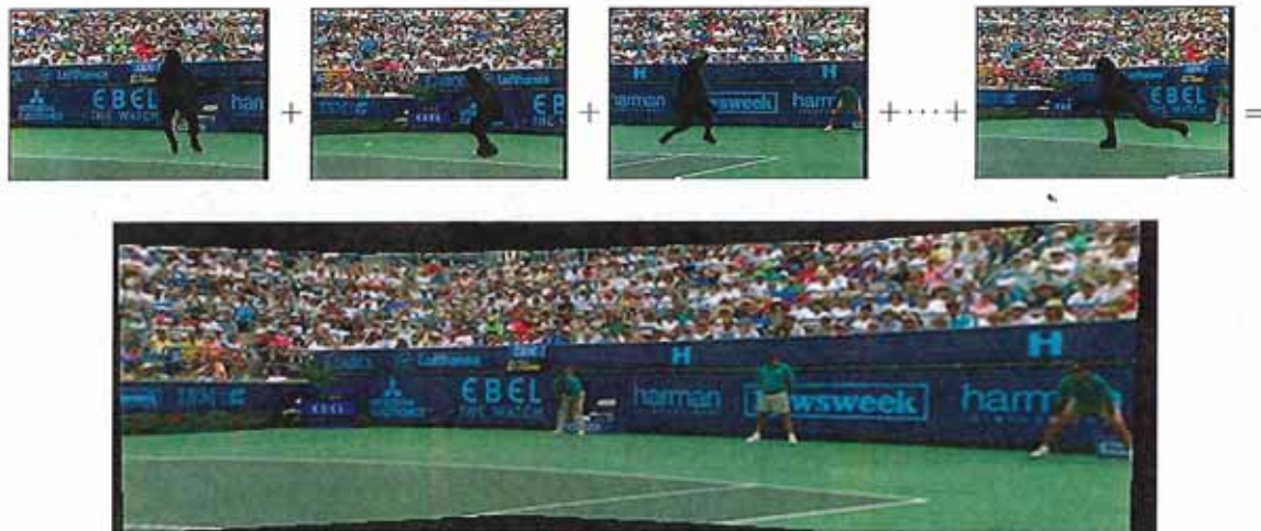
Figure 9.6 Video stitching the background scene to create a single sprite image that can be transmitted and used to re-create the background in each frame (Lee, ge Chen, lung Bruce Lin et al. 1997) © 1997 IEEE.
