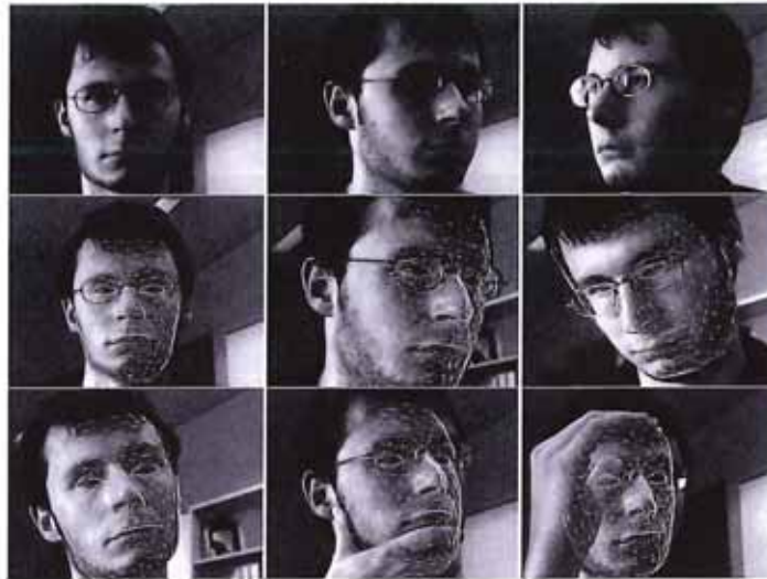
Figure 4.29 Real-time head tracking using the fast trained classifiers of Lepetit, Pilet, and Fua (2004) © 2004 IEEE.
