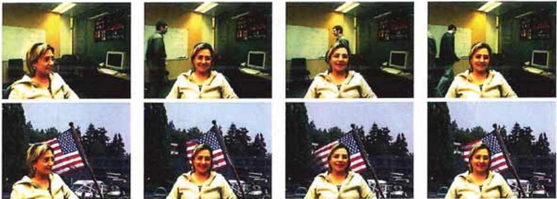
Figure 11.14 Background replacement using z -keying with a bi-layer segmentation algorithm (Kolmogorov, Criminisi, Blake et al. 2006) © 2006 IEEE.
