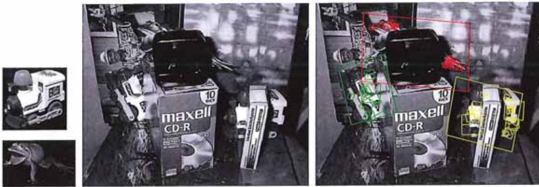
Figure 4.21 Recognizing objects in a cluttered scene (Lowe 2004) © 2004 Springer. Two of the training images in the database are shown on the left. These are matched to the cluttered scene in the middle using SIFT features, shown as small squares in the right image. The affine warp of each recognized database image onto the scene is shown as a larger parallelogram in the right image.
