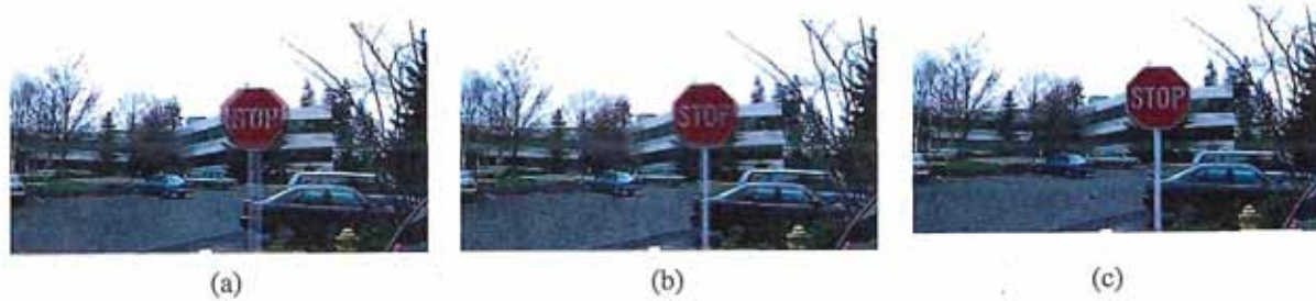
Figure 9.10 Deghosting a mosaic with motion parallax (Shum and Szeliski 2000) © 2000 IEEE: (a) composite with parallax; (b) after a single deghosting step (patch size 32); (c) after multiple steps (sizes 32, 16 and 8).
