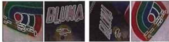
Figure 4.15 Maximally stable extremal regions (MSERs) extracted and matched from a number of images (Matas, Chum, Urban et al. 2004) © 2004 Elsevier.
