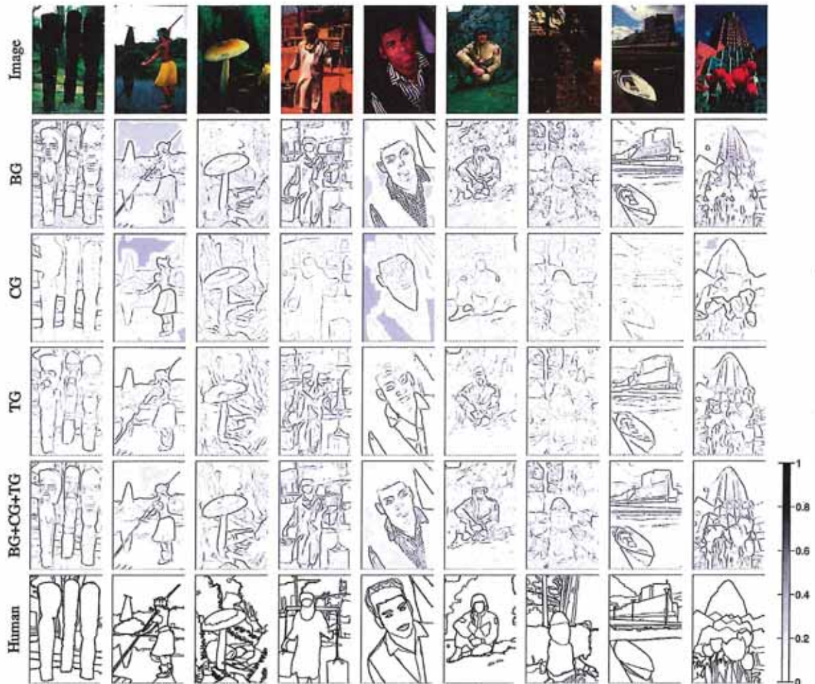
Figure 4.33 Combined brightness, color, texture boundary detector (Martin, Fowlkes, and Malik 2004) © 2004 IEEE. Successive rows show the outputs of the brightness gradient (BG), color gradient (CG), texture gradient (TG), and combined (BG+CG+TG) detectors. The final row shows human-labeled boundaries derived from a database of hand-segmented images (Martin, Fowlkes, Tal et al. 2001).
