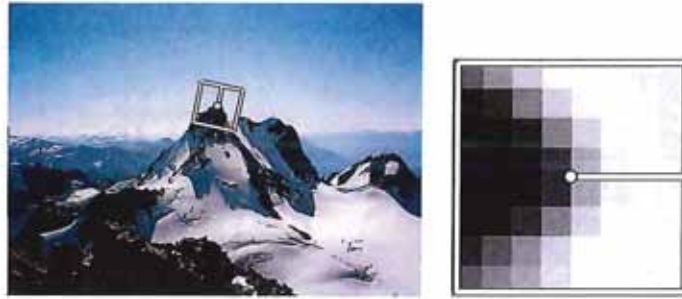
Figure 4.17 MOPS descriptors are formed using an 8 \times 8 sampling of bias and gain normalized intensity values, with a sample spacing of five pixels relative to the detection scale (Brown, Szeliski, and Winder 2005) © 2005 IEEE. This low frequency sampling gives the features some robustness to interest point location error and is achieved by sampling at a higher pyramid level than the detection scale.
