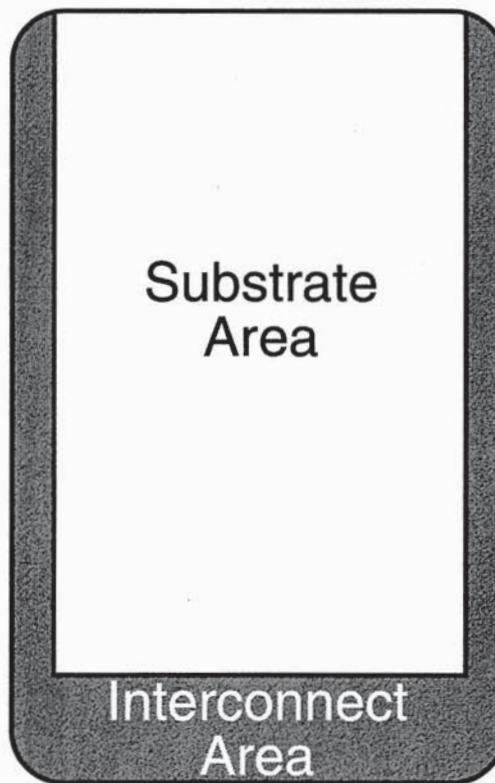
Figure 4-1. The Interconnect Area is the Same Thickness for all PC Cards.
